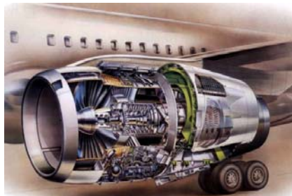
Cut-away diagram of the RB211-535 fitted to a Boeing 757
