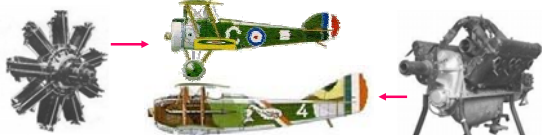
Clerget (Type 11), Sopwith Camel 旋轉式 9缸, 130 hp
